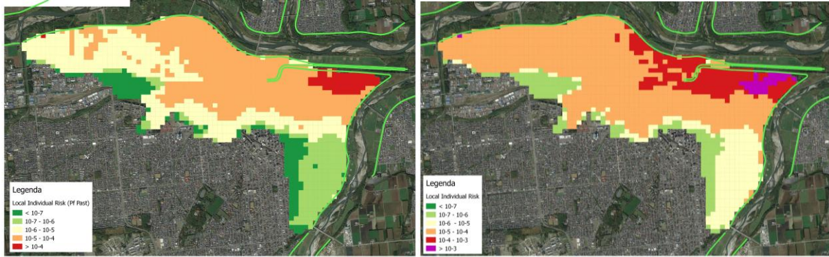
Figure 38 Local individual risk for the "future" situation, 80 percent evacuation, left is the average exceedance probability of the discharges, right is with the 95% upper limit.
