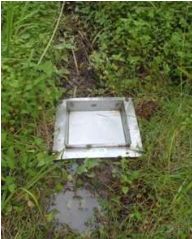
Figure 5. Sediment Trap: Square plates were set on the ground surface in the area. Sediments remained on the plate after inundation.(size: 0.22m×0.22m)
